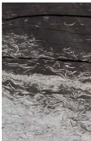
Figure S10. Core photo (oriented) illustrating black shale overlying fossiliferous limestone in Core A.
